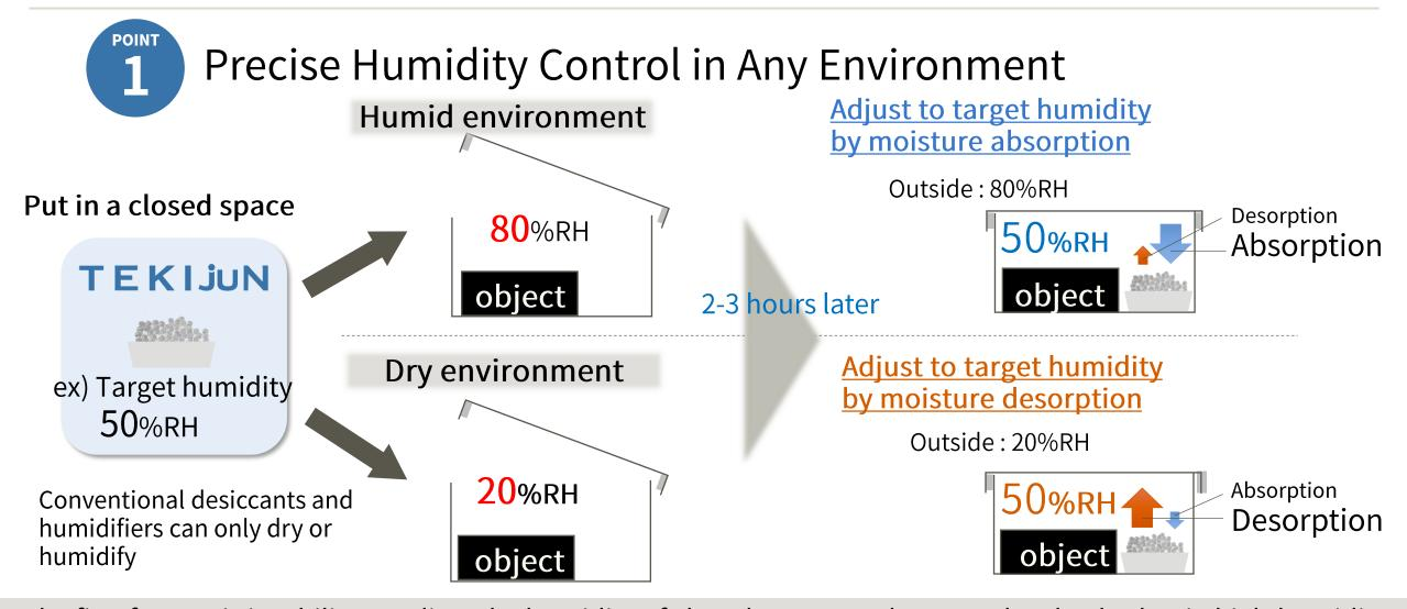
The first feature is its ability to adjust the humidity of closed spaces to the target level. Whether in high-humidity or low-humidity environments, it can regulate the humidity inside a closed space to the desired level by absorbing or desorbing moisture.
