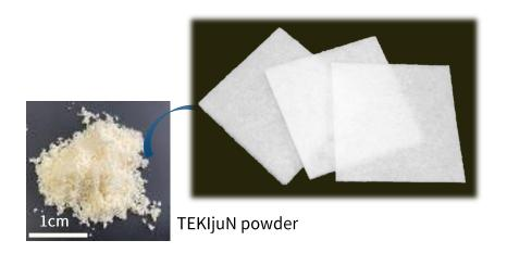
Rapidly absorbs moisture in high humidity, releases and regenerates moisture in low humidity, preventing excessive dryness and humidity.
