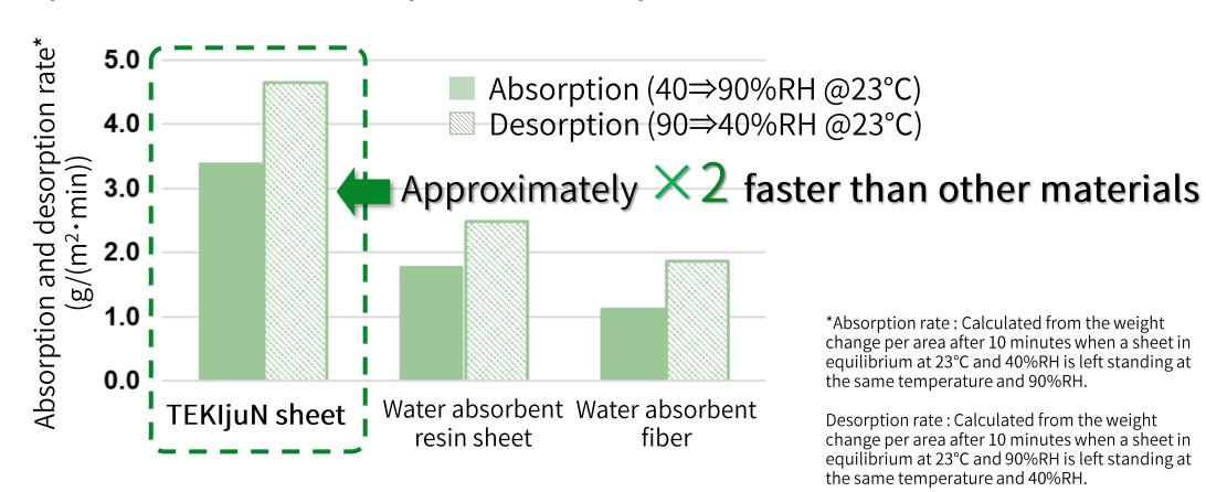
\*Absorption rate: Calculated from the weight change per area after 10 minutes when a sheet in equilibrium at 23°C and 40%RH is left standing at the same temperature and 90%RH.
