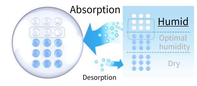
In a dry environment, TEKIjuN releases the moisture it holds, thus increasing the surrounding humidity. On the other hand, in humid environments, TEKIjuN absorbs moisture, resulting in a decrease in the surrounding humidity. This enables precise adjustment of the humidity level inside the closed space to the optimum level.
