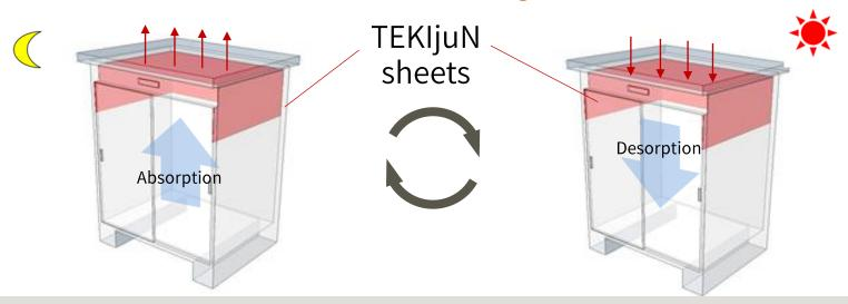
The second feature is its reusability through natural regeneration. After absorbing moisture during high humidity periods, it naturally releases moisture during low humidity periods, eliminating the need for removal and drying.
