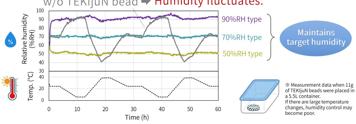
The second feature is its capability to maintain the target humidity even when there are temperature changes. While relative humidity in a closed space increases with decreasing temperature and decreases with increasing temperature, the beads within the closed space ensure that the target humidity is maintained.
