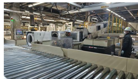
Washing machine conveyor line
