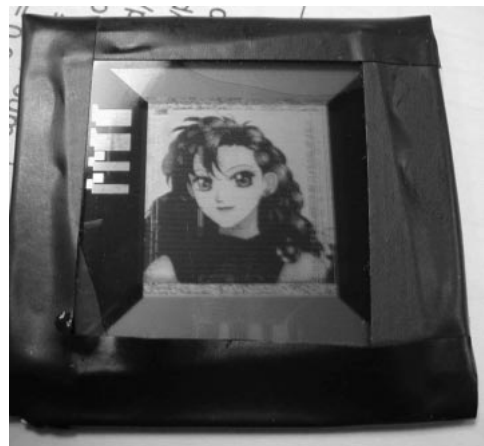
Fig.10 Greyscale is achieved using error diffusion. Interpixel switching gives 95% aperture ratio.
