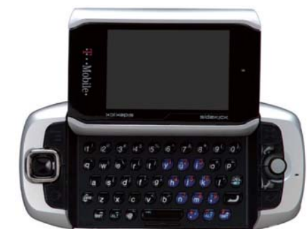
The PV200, or Sidekick III, was lauded for a design that included a trackball for ease of operation
