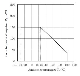
Fig.2 Diode Power Dissipation vs. Ambient Temperature
