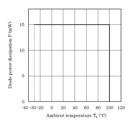
Fig.4 Total Power Dissipation vs. Ambient Temperature
