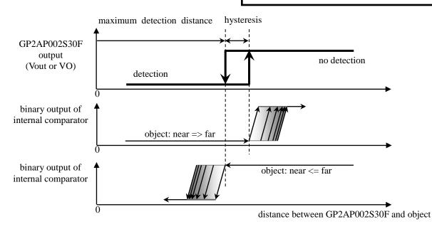
Note that the detection distance can be controlled by changing LED current limiting resistor, too.
