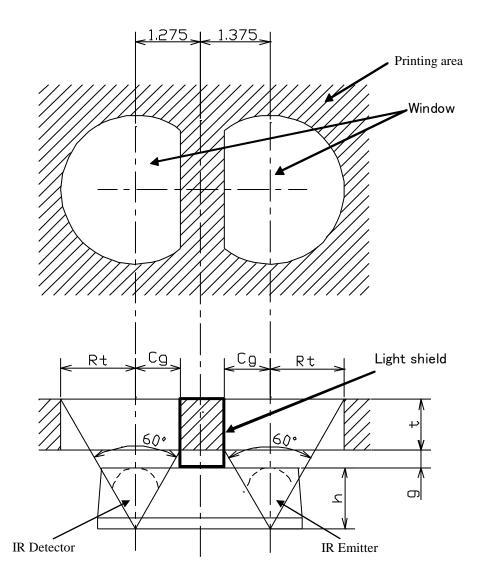
$\begin{array}{ll} h=n \times r \; / \; (n-1) = 1.2 mm \\ n=1.58 & n : mold \; resin \; refractive \; index \\ r=0.45 & r : radius \end{array}$
