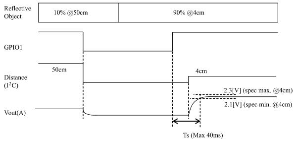
Response time of I<sup>2</sup>C output is faster than that of Vout(A) because it is stabilized soon after distance data output. Distance data is updated every 20ms after response time.
