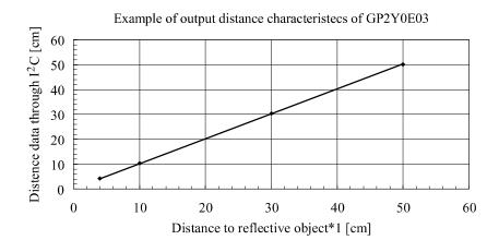
Example of output distance characteristics of GP2Y0E03
