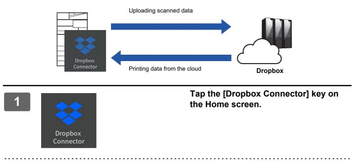
If you cannot find the Dropbox Connector icon on the Home Screen, register the Dropbox Connector to the Home Screen in the Home Screen Settings of the machine System Settings.
