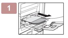
Remove any paper remaining in the bypass tray.
