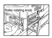
Carefully remove the misfed paper. Turn the roller rotating knob in the direction of the arrow to assist in removing it.
