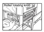
Turn the roller rotating knob in the direction of the arrow.
