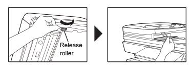
Open the document feeder and rotate the release roller in the direction of the arrow to feed the original out.
