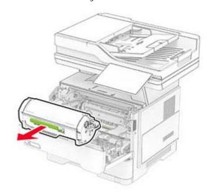
Remove the used imaging unit.
