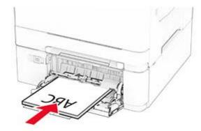
• Load envelopes with the flap side up and against the right side of the paper guide.
