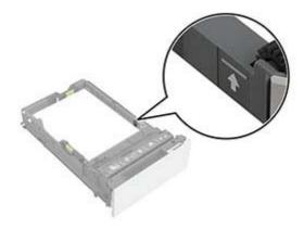
For envelopes and other specialty media, make sure that the stack height is below the dashed line. Overfilling may cause paper jams.
