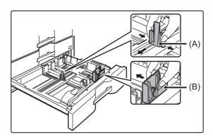
Adjust guide plates A and B by squeezing their lock levers and sliding them to match the longitudinal and transversal dimensions of the paper to be loaded.
