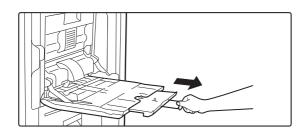
When loading paper larger than A4R or 8-1/2" x 11"R, pull out the extension guide.
