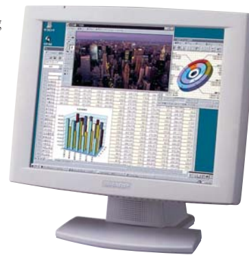
Space-saving CE-LT14M color display using a 13.8-inch Super-V LCD (1997)
