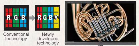
LC-60LV3 AQUOS using four-primary-color technology (2010)
