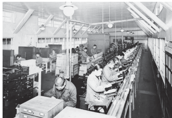
Radio production line using the intermittent belt conveyor system (around 1936)
