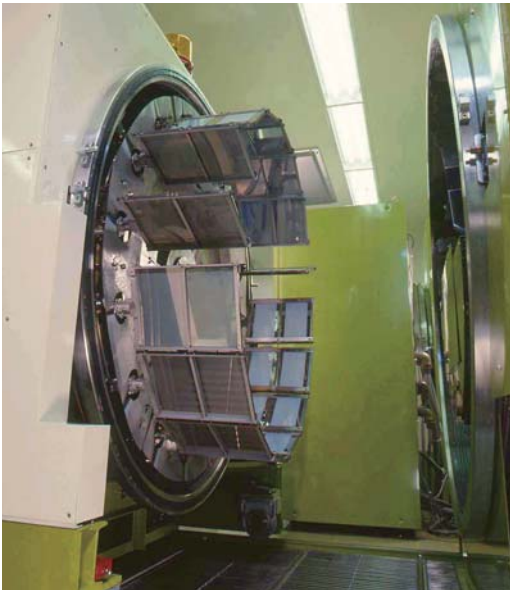
EL panel deposition device that put a thin film coating on a glass substrate by high-temperature vacuum deposition
