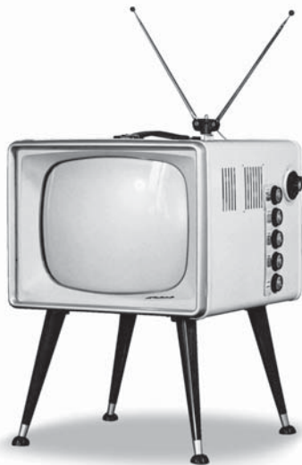
The TM-20 portable TV featured a novel design in which the channel selector and all adjustment knobs were mounted on the side
