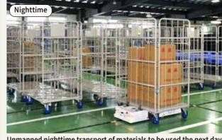
Unmanned nighttime transport of materials to be used the next day from the second-floor warehouse to the first-floor production line
