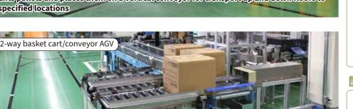
AGVs equipped with conveyor carts dock with the production line conveyor to receive
