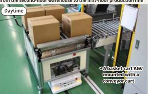
The AGV docks at the conveyor to receive finished products and then automatically transports them to the shipping conveyor.
