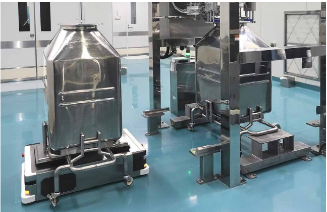
The AGVs repeatedly change and automatically transport containers during the granule container-filling process.
