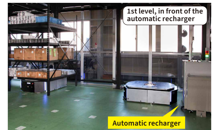
The AGVs automatically transport storage racks and also automatically recharge their batteries.
