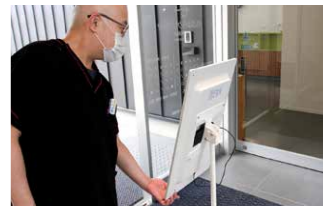
Pressing a button on the rear of the main unit to select the desired display.
