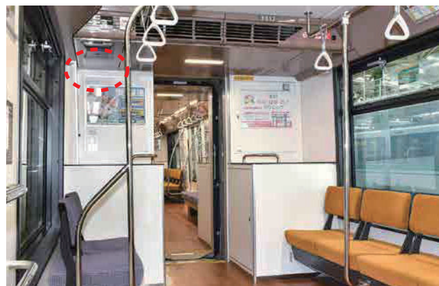
Ions are diffused with a generator installed above seats at the side of the gangway.
