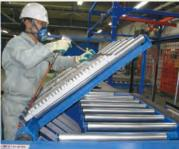
A sloping/reversible workbench makes it easy to remove screws and turn over the flat-panel TVs.
