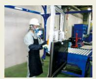
Transfer equipment for large flat-panel TVs ensures minimal burden on workers
