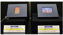
LCD panels incorporating IGZO oxide semiconductor technology
