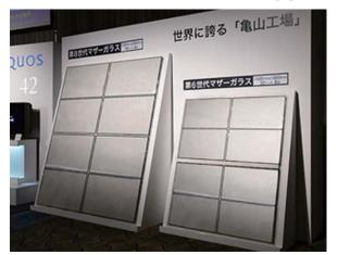
Sixth-generation glass substrate (right) from Plant No. 1 and eighth-generation glass substrate (left) from Plant No. 2, which started operations in August 2006
