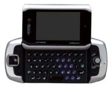
The PV200, or Sidekick III, was lauded for a design that included a trackball for ease of operation
