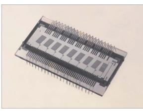
Prototype of LCD used for electronic calculators (1972)
