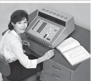
The CS-10A, the world's first all-transistor diode electronic desktop calculator
