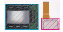
A System LCD (right) has fewer peripheral components and requires a smaller mounting area (shown with diagonal lines) than conventional LCDs. The photographs provide a comparison for LCDs used in projectors.
