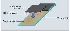
In a Blacksolar PV cell, the silver electrode and copper wiring are directly connected, and the line width is thicker, reducing the loss of generated power (schematic diagram)
