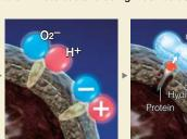
2. lons decompose mold fungi and bacteria When Plasmacluster lons come into contact with the surfaces of mold fungi and viruses, they turn into highly oxidizing hydroxide (OH) radicals that instantly remove hydrogen (H) from surface proteins, breaking them down.
