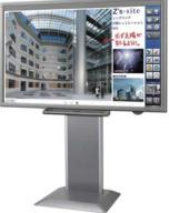
Sharp aimed to generate new demand with the 80-inch PN-L802B touchscreen LCD monitor. It gave this large display the nickname BIG PAD in Japan. (January 2012)
