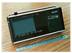
Prototype 3.2-inch TFT color LCD TV (1985)
