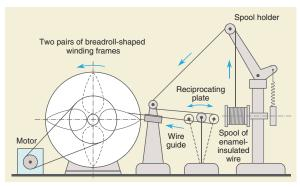
Deflection coil (top) and operation of deflection coil winding machine (bottom)
