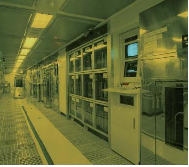
Microfabrication processing line for color TFT LCDs (Tenri Plant)
