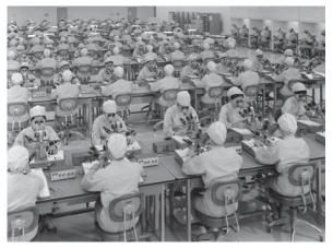
Employees at the semiconductor plant working with microscopes in the later stages of the production process
