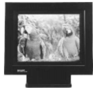
Photo 8 The first large (14") TFT-LCD.
