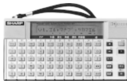
Photo 3 An electronic translator with an alphanumeric LCD.
