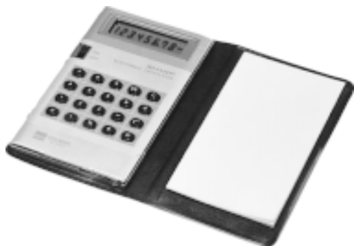
Photo 2 A portable calculator with a TN-LCD EL8020.
