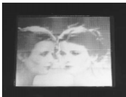
Photo 4 A 5.5" B/W LC-TV with a XY matrix LCD (160 x 120 dots).
