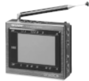
Photo 7 The first LC-TV product using a-Si TFT-LCD from SHARP.
