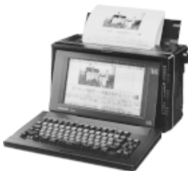
Photo 6 The first B/W LCD word processor using a doublelayered STN-LCD.
