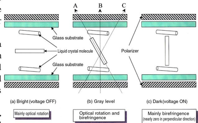
Fig. 1 The principle of TN mode.
