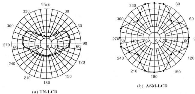
Fig. 7 The viewing angles of normal TN and ASM mode.<sup>7)</sup>
