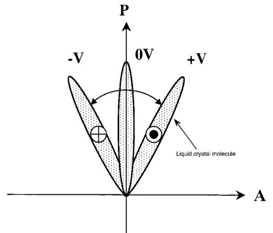
Fig. 12 The principle of monostable FLC showing full gray scale.<sup>14)</sup>
