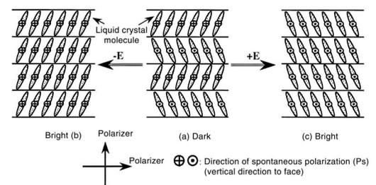
Fig. 13 The AFLC showing full gray scale.<sup>17)</sup>
