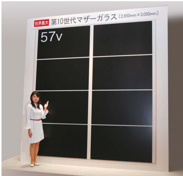
10G glass substrate employed at the new LCD panel plant
