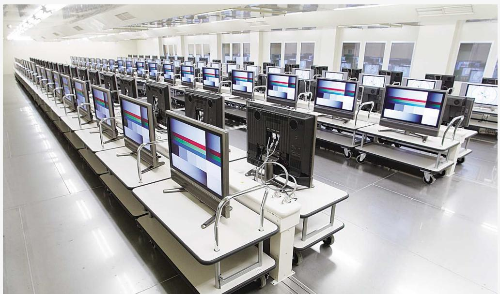
LCD TV production line (isothermal test process)
