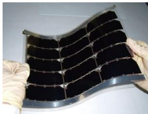
Ultralight flexible solar cells
