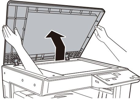
The automatic document feeder (BP-20M22/BP-21M22/BP-20M24/BP-20M28/BP-20M31) cannot be removed.
